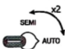
TURN THE SELECTOR TWICE FROM AUTO TO SEMI. AND ENTER THE PROGRAM SELECTION IN "SEMI" MODE. LONG PRESS THE TRIGGER UNDER "AUTO" MODE FOR THREE SECONDS TO SAVE THE PROGRAM.
